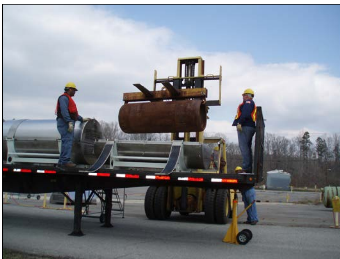
UF_6 cylinder being loaded for transport at ETTP
