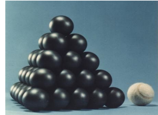
graphite SNF spheres
