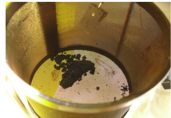
Recovered Fuel from Digested Graphite Sphere
