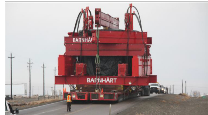
1,082-ton packaged PRTR being transported to ERDF for disposal
