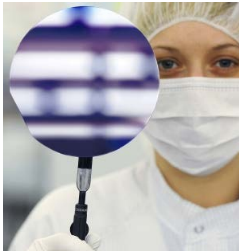
Figure 2.6 GaN-based LEDs on a 200 mm Silicon Wafer as Demonstrated by OSRAM
