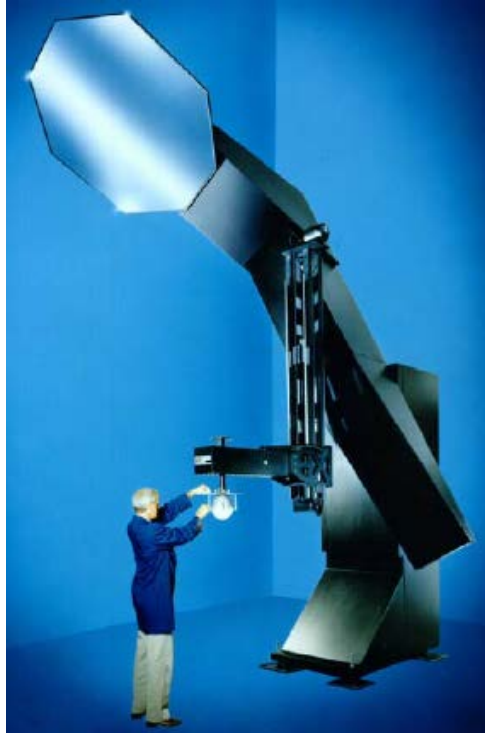
Figure 2.5 High Speed Moving Mirror Goniophotometer Model 6400 T by Lighting Sciences Inc.
