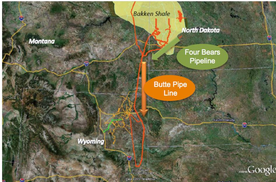
From these points, Bakken crude can travel our Butte Pipe Line to major interstate pipeline connections at Ft. Laramie and Guernsey, WY, or by rail to customers across the country. With a capacity of 110,000 barrels per day, we estimate that construction of the Four Bears Pipeline took over 300 trucks per day off of US Highway 85 and ND Highway 22. This translates to over 25 million truck miles off the roads in North Dakota.
