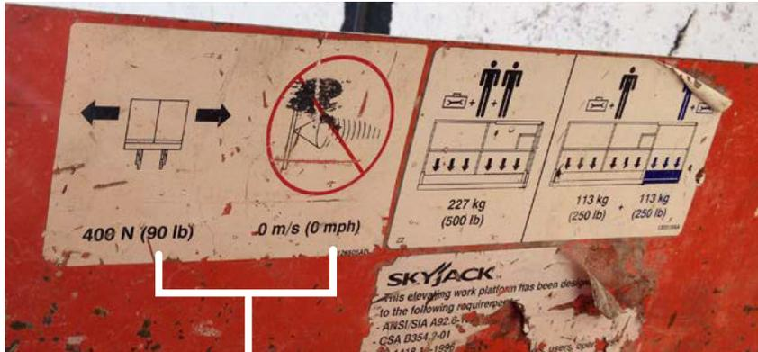
**Figure 1-6. Manufacturer-applied label shows 0 mph wind and 90 lb side force limitations**
