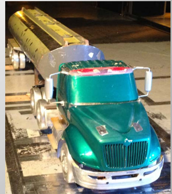
Performed extensive wind tunnel tests at Army 7x10 facility in the NASA Ames Research Center
