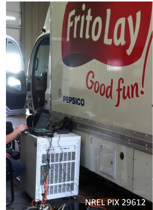
Battery Degradation Load Test Setup
