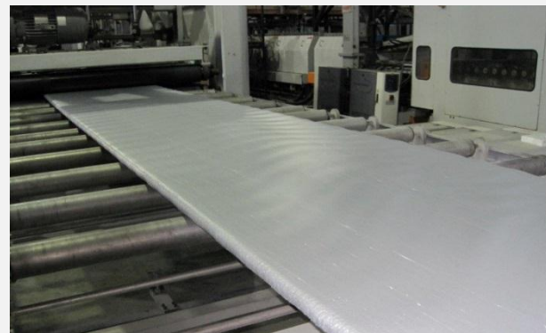
© ISTN XPS board produced in factory demonstration
