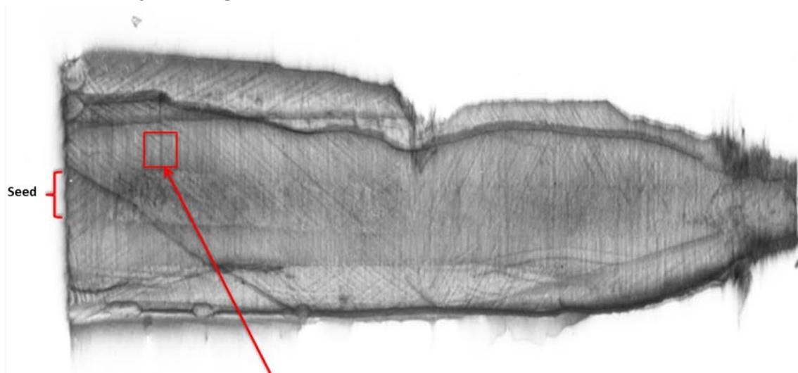
Abundance of defects observed propagating from seed crystal defects.
