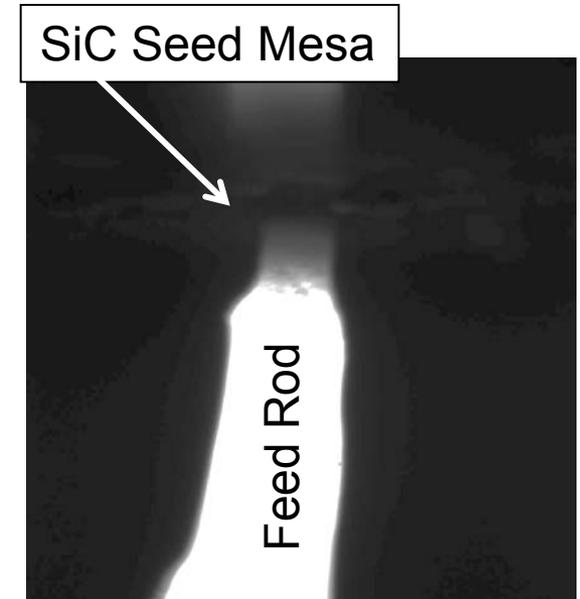
Melted feed rod tip successfully wetted to single hexagonal patterned SiC seed mesa.
