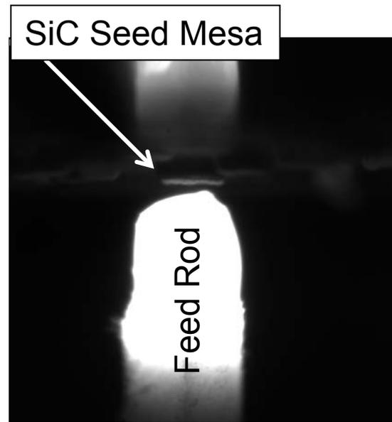
Melt formed on tip of feed rod just prior to contact with patterned SiC seed mesa.
