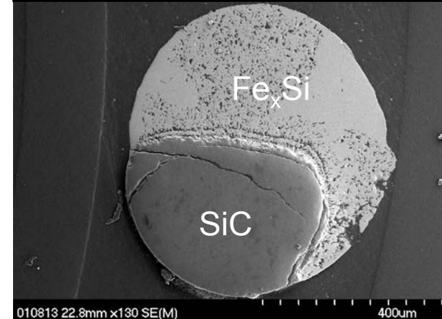
Cross sectional SEM image & EDS elemental analysis of successful extrusion and sintering of Si-Fe-graphite feed rod (sample embedded in epoxy)
