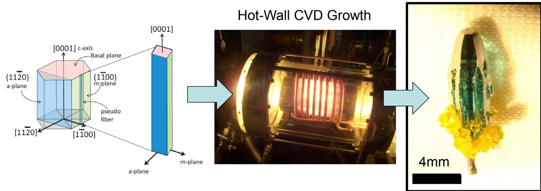
A 4 mm diameter 4H-SiC “mini-boule” was grown using this process during FY12, but sample exhibited abundant parasitic 3C-SiC growth in region where sliver is held by graphite carrier.
