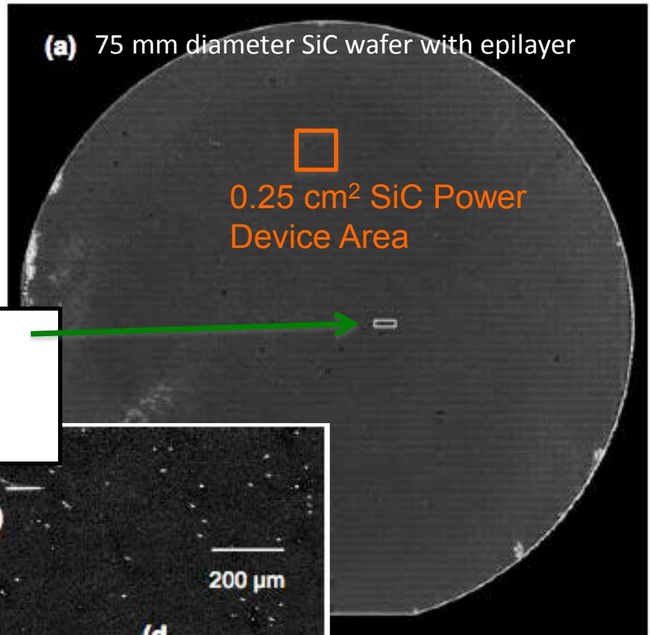
Magnified view small area in middle of wafer imaged by Ultra-Violet Photoluminescence
