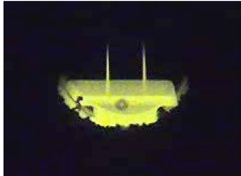
Thermal image of TaC-coated carrier and 4H-SiC seed slivers inside NASA hot-wall CVD reactor during  $T > 1400^{\circ}\text{C}$  pre-growth  $\text{H}_2/\text{HCl}$  etch.
