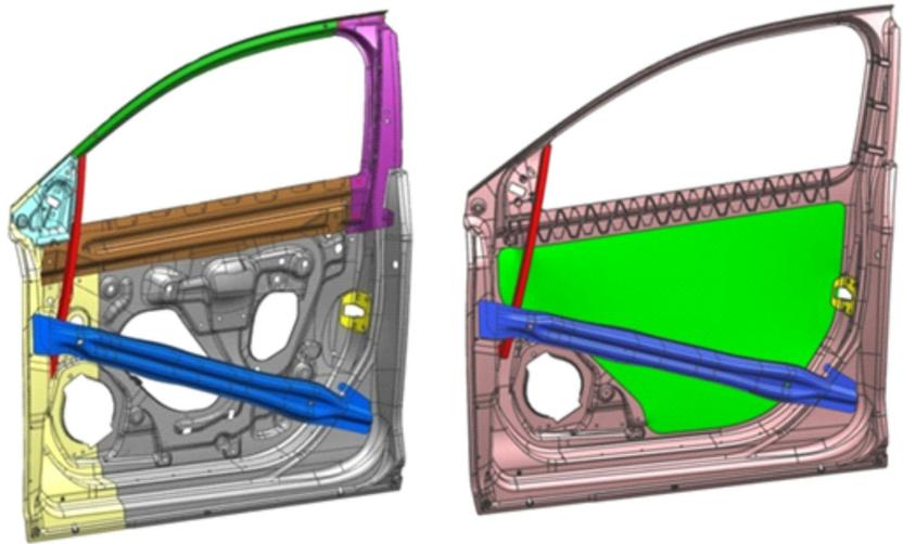
The magnesium door inner produced during this project (right) will be cast to shape, compared to an equivalent steel stamped door inner (left), which is made of multiple pieces that must be welded, thus requiring additional manufacturing steps.
