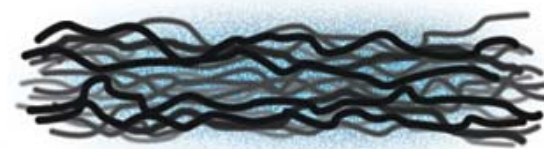
Chain orientation in drawn polymer
