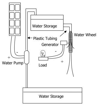
**Suggestions:** Try connecting the load directly to the PV panel, and then try connecting the load through the water wheel generator. Which way works the
