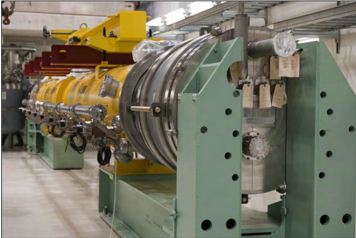
Figure 2-4 Typical Cryomodule (yellow) Portion of a Linear Accelerator
