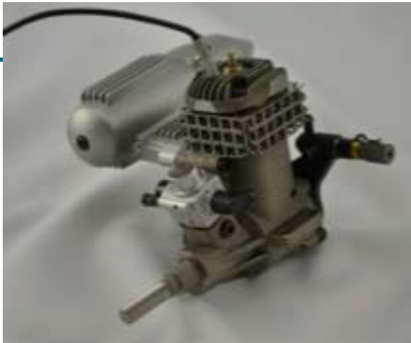
Titanium engine head and block printed by the ORNL Additive Manufacturing team. AM enabled a pressure sensor port to be printed in (shown with sensor installed)
