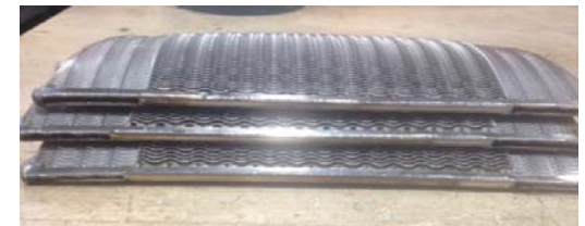
8" AFA air cells (~90 made) for rainbow recuperators
