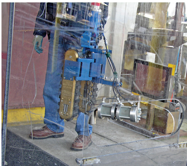
Exhibit 4-13: Box for Crawler Sampling and Repairs
