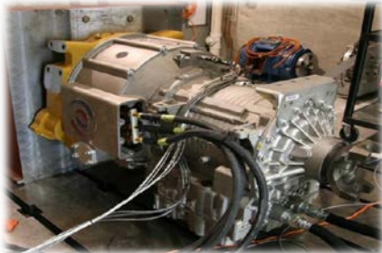
High Voltage Onboard Generator w/ Transmission
