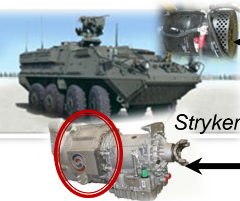
Stryker High Voltage Onboard Generator
