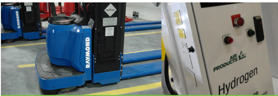
Left: Class III fuel cell powered lift truck at Sysco Houston distribution center in Houston, TX. Sysco Houston . Right: Indoor refueling station for fuel cell powered lift trucks at FedEx Freight East facility in Springfield, MO. FedEx Freight East .
