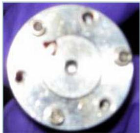
three screws was inconsistent with the safety review expectations and posed an increased risk of the canister seal failing (Figures 2-1 and 2-2).
