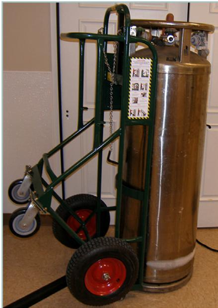
**Figure 1-3. Non-DOE Dewar and cart in pre-tipped configuration**
