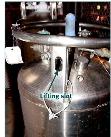
Figure 1-2. Dewar lifting slot
