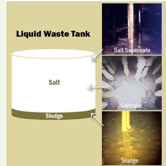
A liquid waste tank and its separate components
