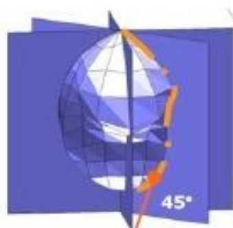
Tri-dimensional candela distribution curve at 45°
