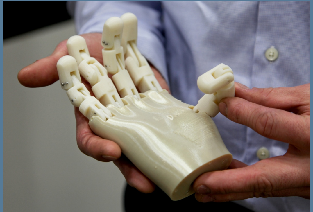
Robotic hand fabricated at Oak Ridge National Laboratory using additive manufacturing technology
