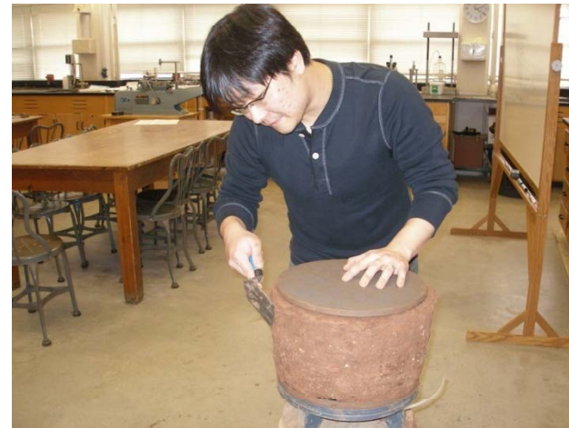
Trimming to the pedestal size
