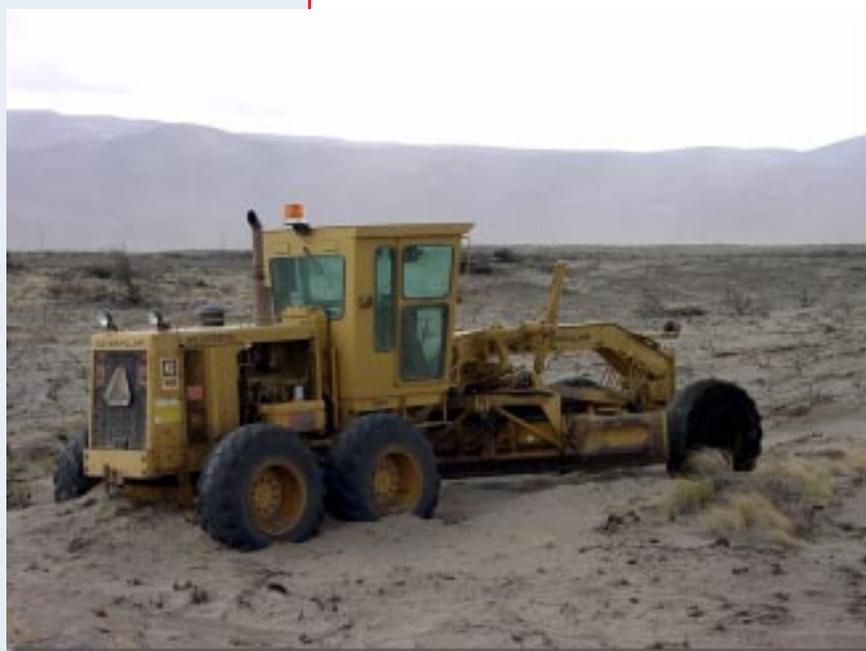
A road grader became stuck in soft sand while grading a firebreak west of the Rattlesnake Barricade. Because of rapidly approaching fire, the operator abandoned the grader and moved to safety with no injuries. Fire damage to the road grader was limited to the front section.
