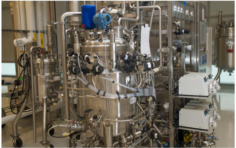
The Advanced Biofuels Process Demonstration Unit at LBNL can convert biomass into advanced biofuels in sufficient quantities for engine testing. *Photo: LBNL*
