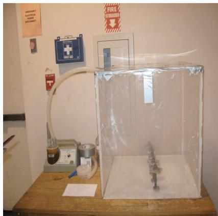
Figure 6. The salt mist spray corrosion testing chamber.
