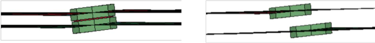
Figure 8. Lap shear test simulation for small spot weld nugget diameter (4.3 mm). DP780 steel.
