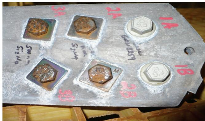
Figure 9. Steel fastener/Mg assemble corrosion test conducted at the GM corrosion laboratory after the first testing cycle. The left four are steel fasteners after silicon nitride coating, the right two are GMW3359 (organic Zn-Al coating) which is showing galvanic corrosion.
