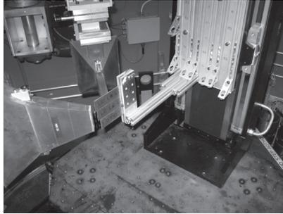
Figure 3. Experimental setup for neutron diffraction stress measurement in the normal direction perpendicular to the plate.
