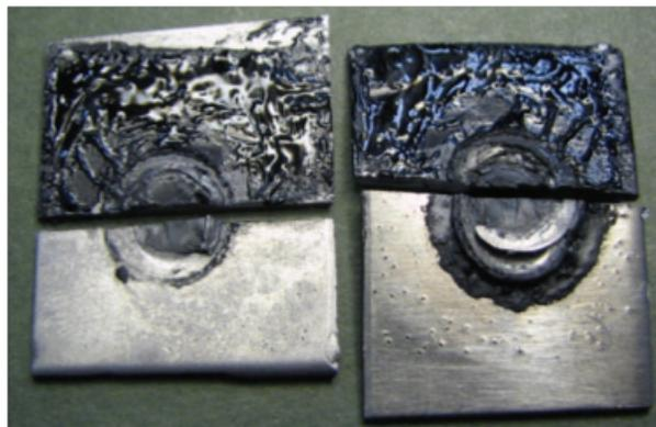
Figure 14. Close view of adhesive after tensile test of FBJ. Initial Figure of Merit Comparison and Analysis
