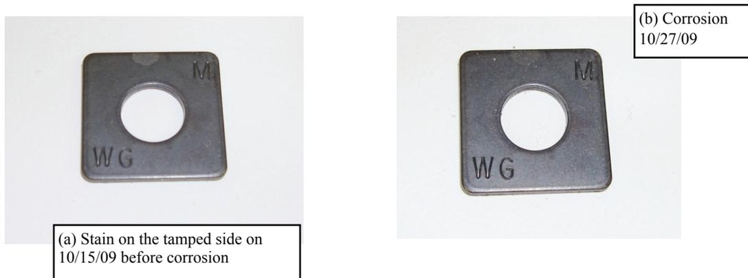
Figure 10. SiN coated steel washer after 12 days in the environmental chamber. First corrosion always showed in the area where stains are.
