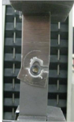
Figure 5. Failure of AA5753 base metal sheet during lap-shear tensile test of a DP980/AA5754 FBJ specimen.
