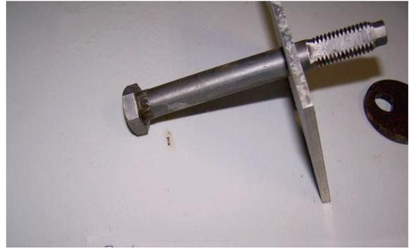
Figure 8. Overall of the M14 fastener after 21 days
