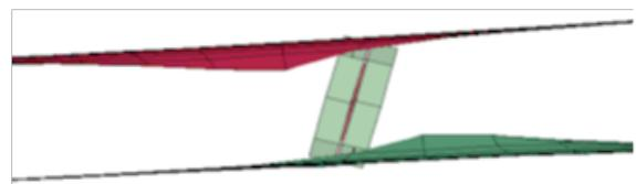
[Figure 10](#). Lap shear test simulation for large spot weld diameter (5.9 mm).
