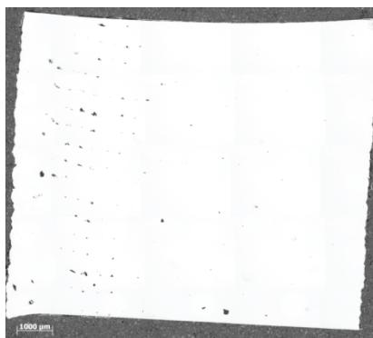
Figure 3. Cross-section of Sample 2 showing that pores appear to have a regular distribution.
