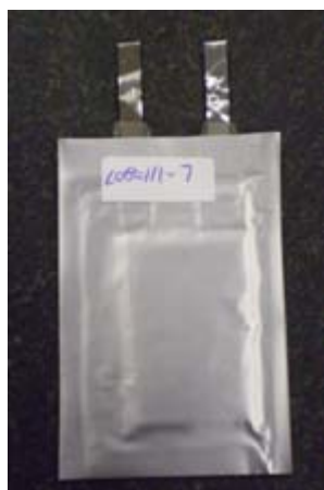
Figure III - 36: GEN 1 35 F lab cells delivered to INL for testing.
