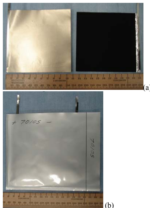
Figure III - 80: a) Anode and cathode with terminals; b) 2.5 Ah cell.
