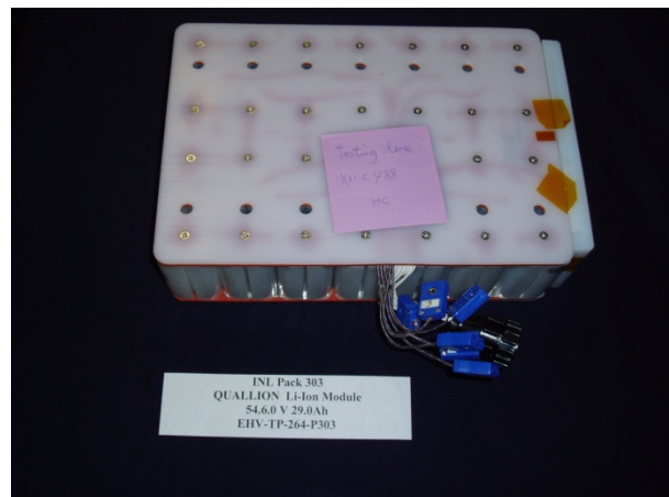
Figure III - 134: Quallion Li-Ion Module
