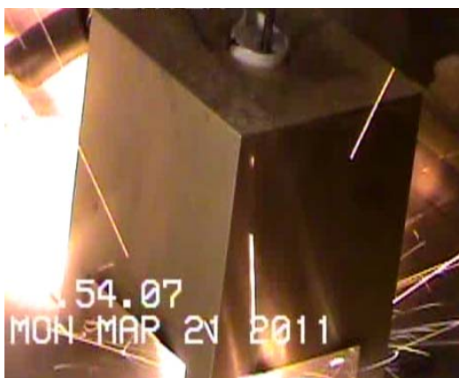
Figure III - 162: Still photograph of cell shorting and runaway during the axial blunt rod test
