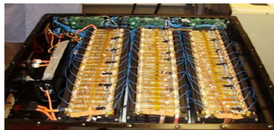
Figure III - 19: Bench test system (internal build) for thermal validation.
