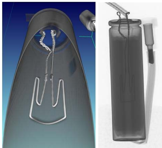
Figure III - 159: CT image (left) and 2D x-ray image (right) of lithium-ion cells built with internal heaters
