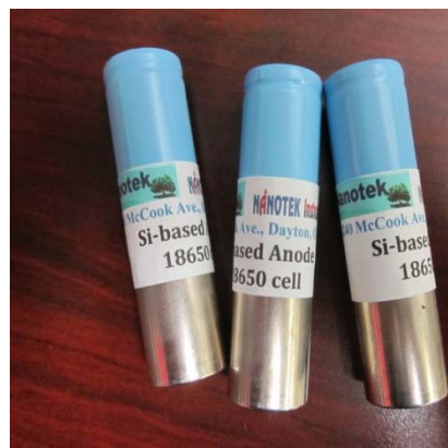
Figure III - 88: 18650 type cells made of Silicon/CNF/graphene platelet based anode and \text{LiFePO}_4 cathode.
