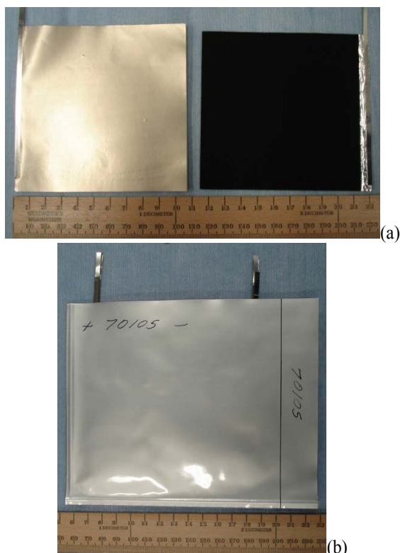
Figure III - 108: a) Anode and cathode with terminals; b) 2.5 Ah cell.
