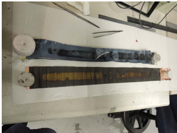
Figure III - 208: E-One Moli 18650 cathode and anode assemblies unrolled after ISC activation.
