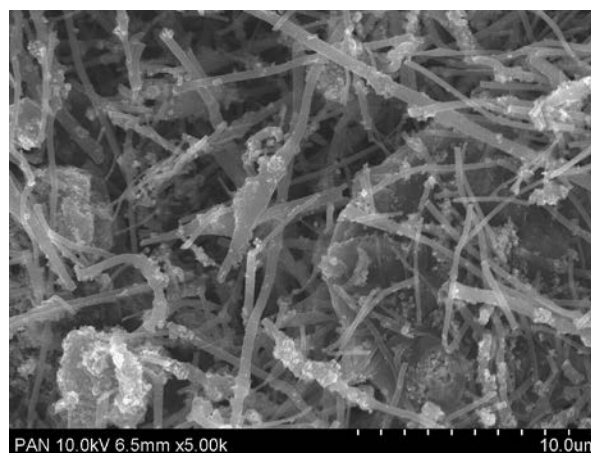
Figure III - 118: SEM image of SiNP/CNF-30-2.
