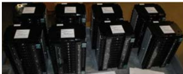
Figure III - 168: Photo of the JSR Micro LIC Modules.
