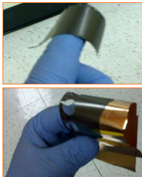
Figure III - 79: Flexible free-standing dry process anodes have been fabricated and laminated to copper current collectors.
