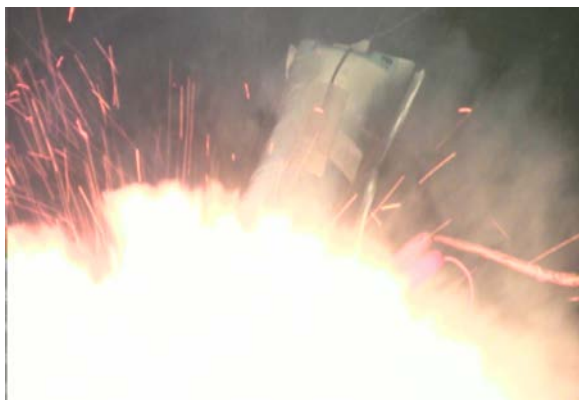
Figure III - 188: Venting and ignition of COTS Li-ion cell contents during overcharge abuse test.
