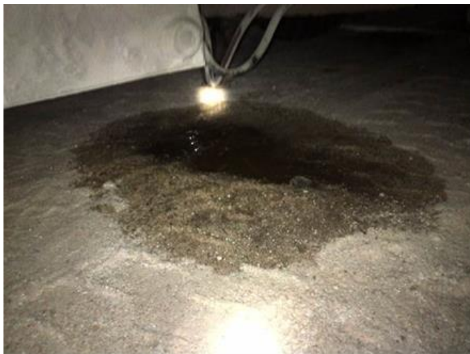
Figure 14: Hydraulic Fluid under Truck 74U006A
