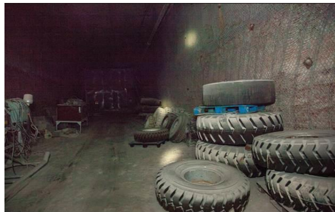
Figure 17: Combustible Loading in the Mine
