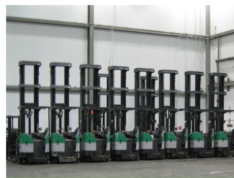
Fuel cell powered lift trucks at H-E-B Grocers in San Antonio, Texas.
