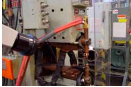
Figure 1: IR imaging of resistance spot welding.
