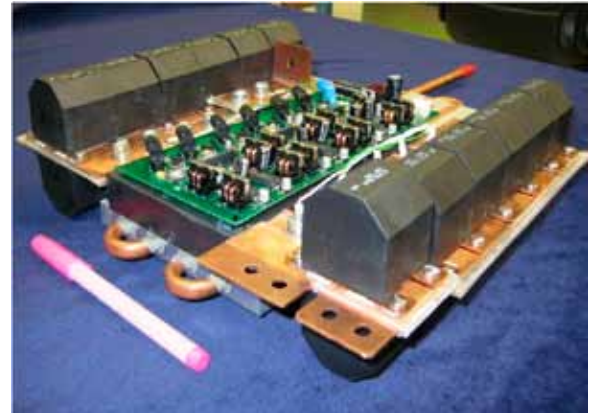
Figure 1: Prototype 55 kW dc-dc converter.
