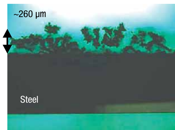
Figure 9. Photograph of deposit layer in surrogate EGR cooler tube. Thermal conductivity found to be essentially that of air, hence loss of heat transfer effectiveness.
