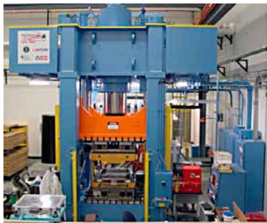
Figure 2: ORNL press and mold for evaluating preform developments.
