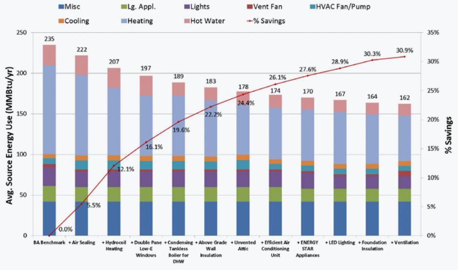
CARB used the National Renewable Energy Laboratory's BEopt energy simulation software to analyze each of the energy efficiency measures for optimized whole-building performance.
