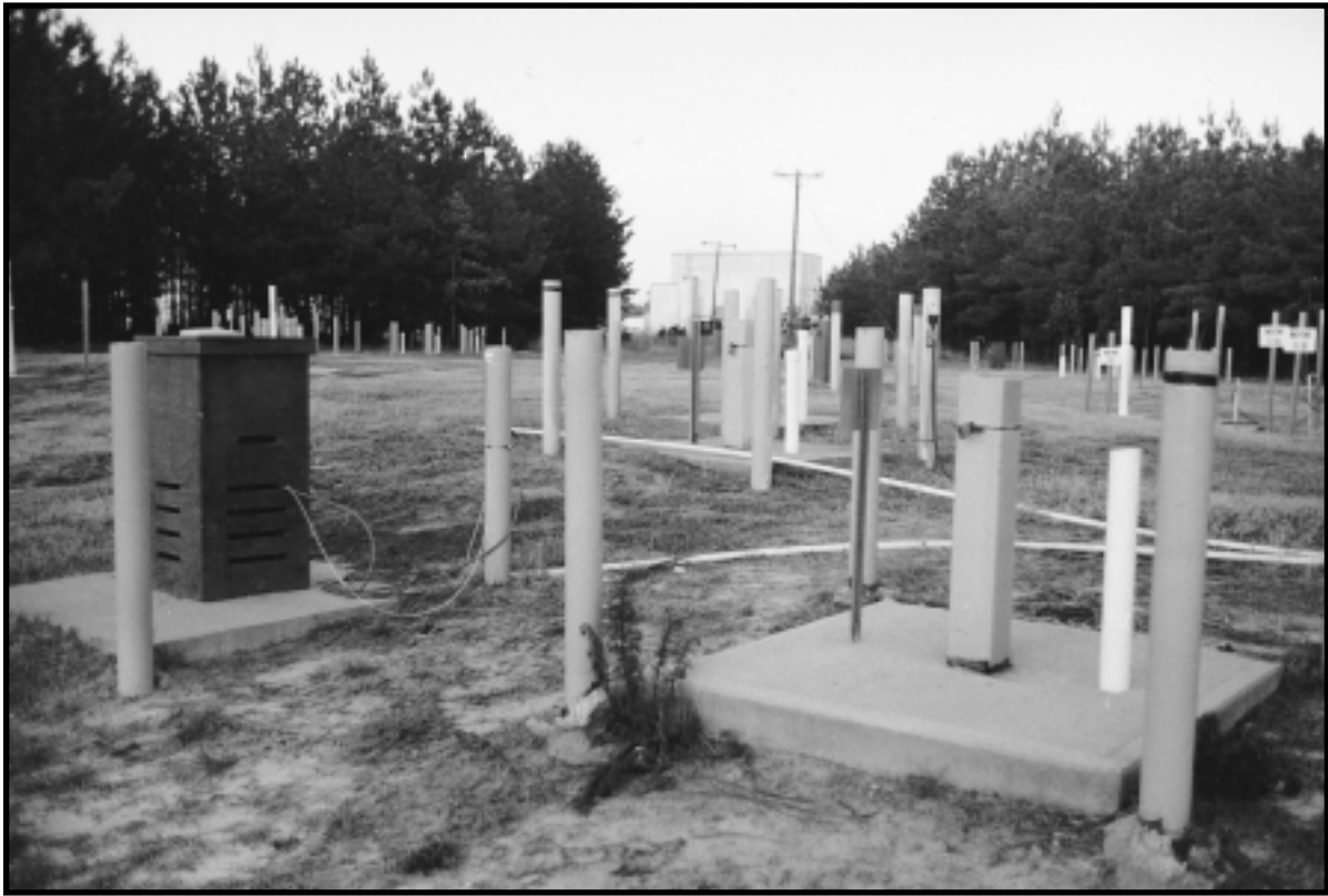
Field of Wells at Savannah River Site A-M Area. The Integrated Demonstration site contains 150 monitoring wells, some quite shallow and some as deep as 200 feet. The wells keep track of the contamination left after the major cleanup project at the M Area, which included removing large amounts of waste, capping the old disposal area, and pumping and treating contaminated groundwater. The site also includes the world's first horizontal injection well used for environmental remediation. M Area Settling Basin, Savannah River Site, South Carolina, January 1994.
