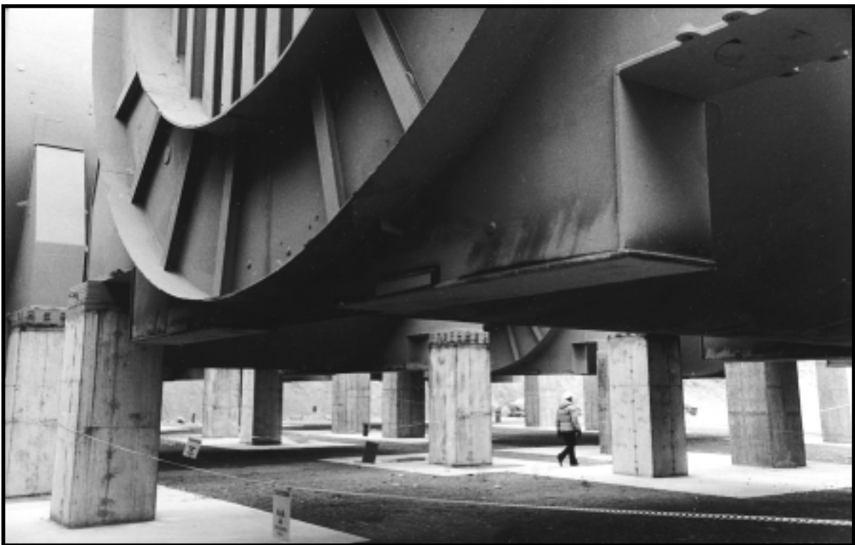
Submarine Hulls Up Close. Use of the thick steel submarine hull as a disposal container provides extra isolation between the environment and the low-level waste and hazardous lead that remain after the spent nuclear fuel has been removed. Trench 94, Hanford Site, Washington, July 1998.
