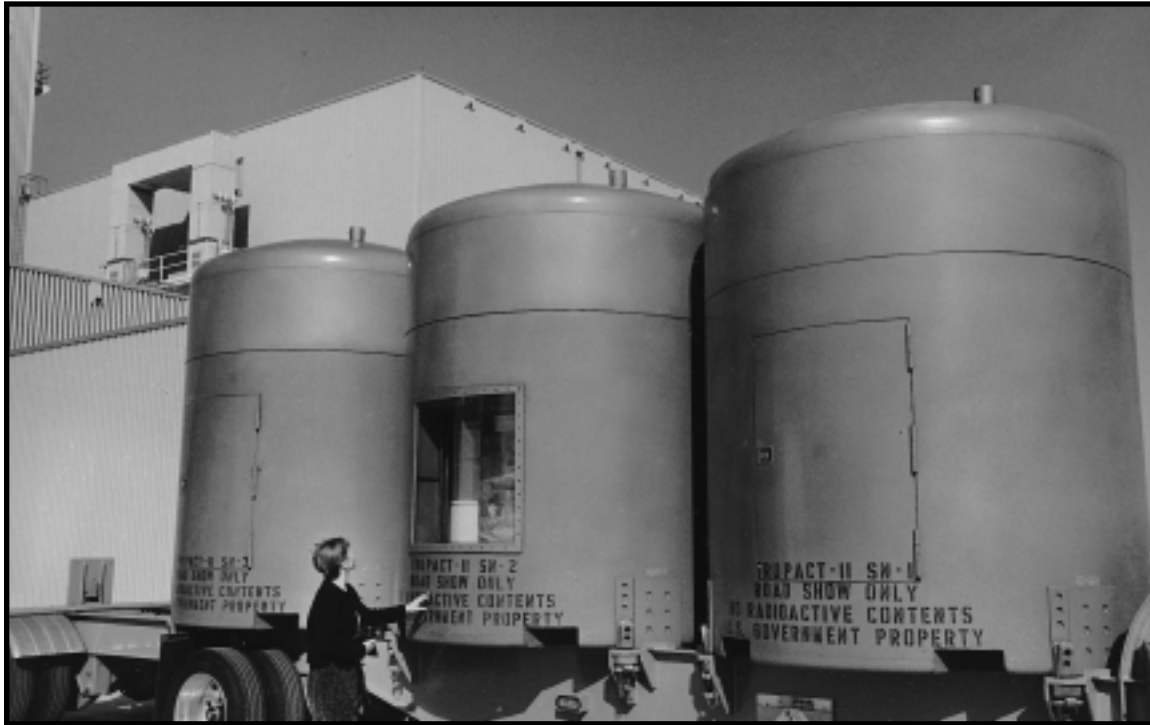
Special Casks for Shipping Transuranic Waste. These demonstration models are similar to those being used to ship transuranic waste to the Waste Isolation Pilot Plant in New Mexico. Each of these Transuranic Package Transporter (TRUPACT-II) casks can hold fourteen 55-gallon drums. A window in the center model cask shows mock waste drums cut open to reveal typical constituents of transuranic waste. Waste Isolation Pilot Plant, New Mexico, February 1994.
