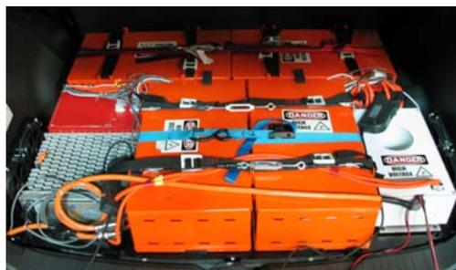
**Figure 3. Inside the Electrovaya Escape PHEV Battery System**
