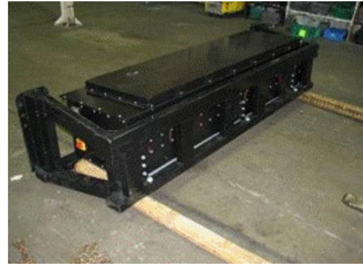
**Figure 4. Enova PHEV Battery Pack**
