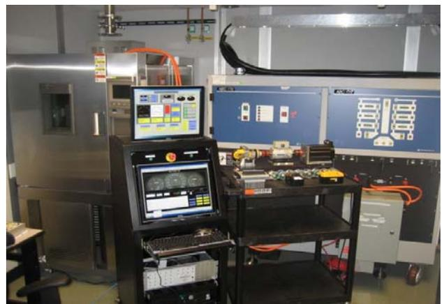
Figure 9. Argonne Battery Hardware-in-the Loop Test Facility
