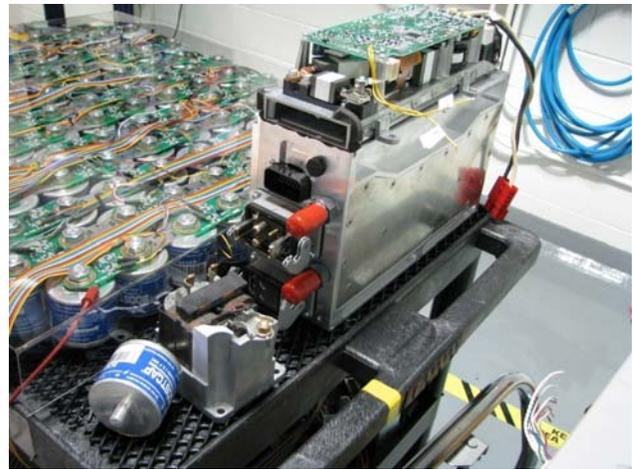
**Figure 11. 60-kW (peak) Brusa BDC412 DC/DC Converter.**
