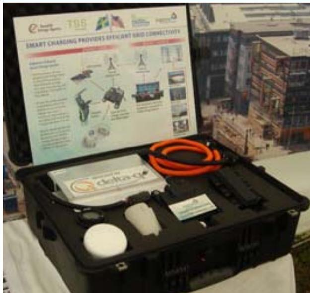
**Figure 11. Argonne-Designed Smart Charging System for a PHEV**
