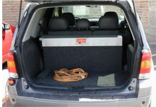
**Figure 7. A123 Lithium Ion Battery Pack Placement in the Hymotion conversion of a Ford Escape: The pack sits close the back site of the Escape in the rear storage area. A PHEV suitable charging infrastructure extension cord is in the back storage area. The pack is topped by the silver colored metal**
