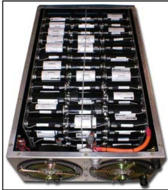
**Figure 10. Maxwell Ultracapacitor Pack**
