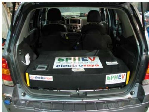
**Figure 2. Battery System of the Electrovaya Escape PHEV**
