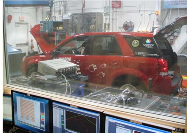
**Figure 22. Saturn TTR PHEV undergoes testing on Argonne’s 4WD Chassis Dynamometer**
