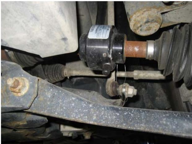
**Figure 5. Axle Torque Sensor**
