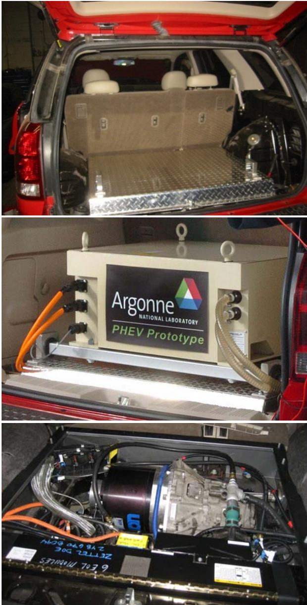
Figure 7. Through-the-Road Parallel Hybrid Powertrain Design Detail
