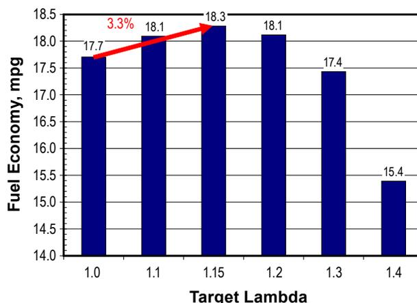
FIGURE 2. Fuel economy on hot-start city tests versus target lambda.
