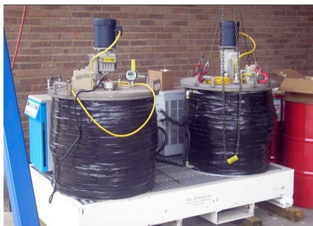
**FIGURE 3.** Stir Tanks Being Used for Materials Compatibility Testing
