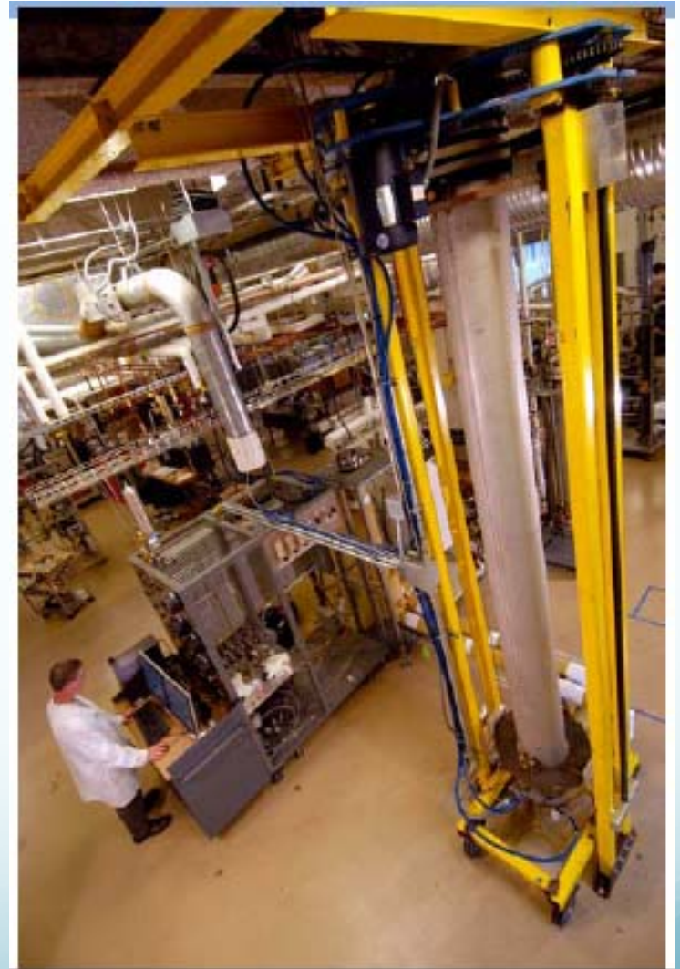
RTI's Transport Reactor System
