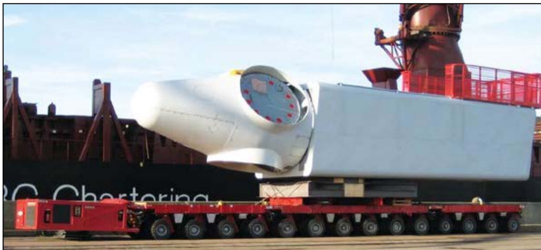
Figure 5-7: Nacelle on Trailer of Self-Propelled Modular Transporters
