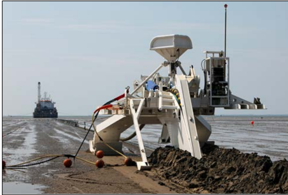
Figure 3-13: Subsea Cable Plow Burying Cable at Shore
