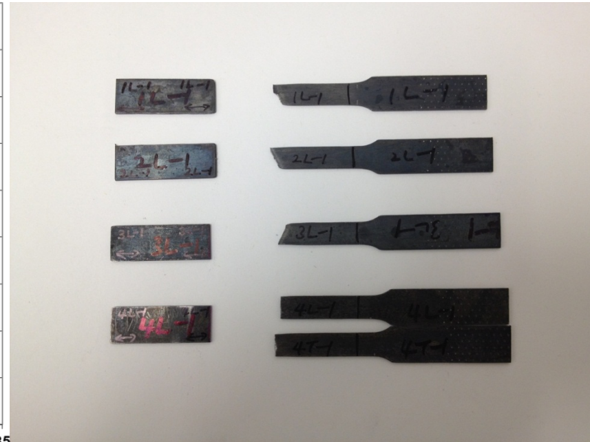
Comparison of tensile failure modes
