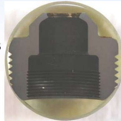
Cross section of undamaged nozzle (material: type 440C)
