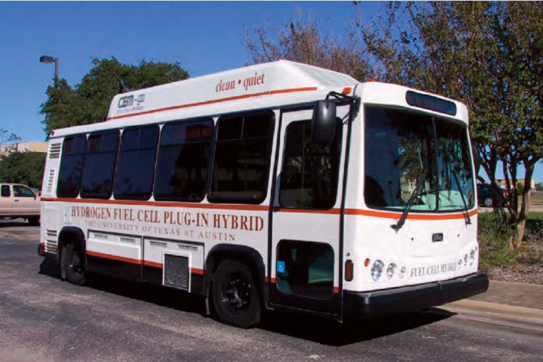
E-bus: 22-ft fuel cell electric battery plug-in hybrid bus in Austin, Texas
