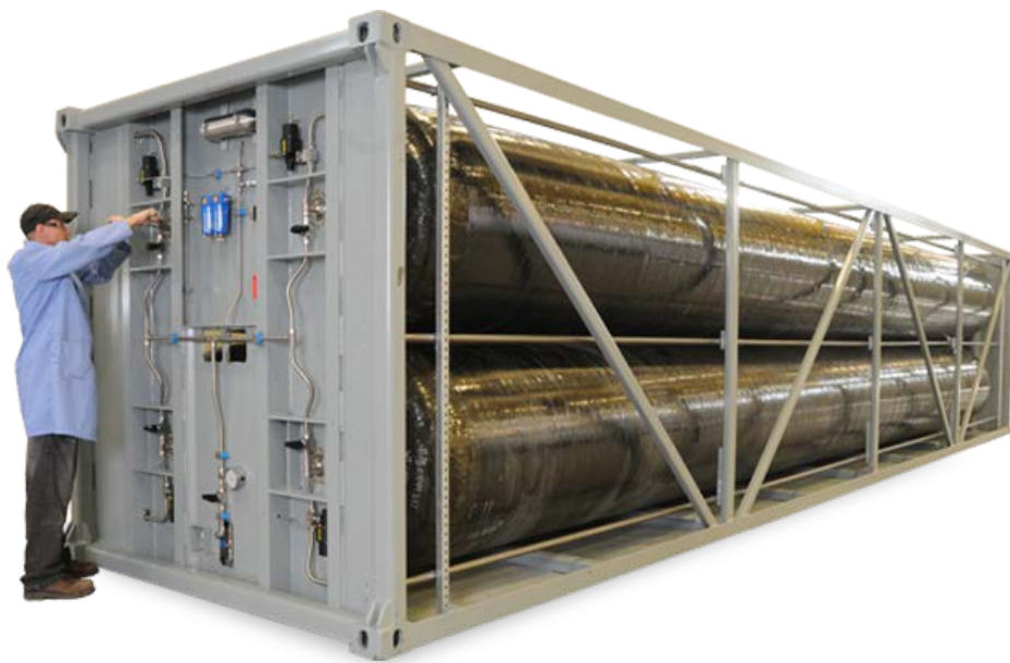
Figure 3-2: The TITAN gas storage module from Lincoln Composites, in the profile of a standard 40-ft shipping container, which can hold approximately 625 kg of hydrogen at 3,600 psi (250 bar) [68].
