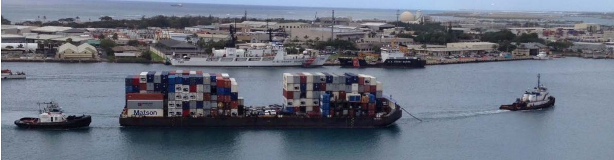
Figure 3-6: Short voyages between neighbor ports, for example the inter-island transports in Hawaii shown here, often utilize container-laden barges pulled by tugs.
