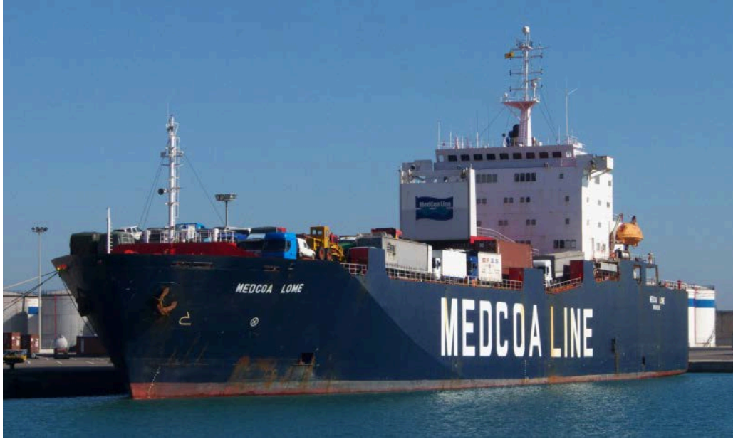
Figure 2-2: The Medcoa Lome (IMO 8508369) RoRo carrier, 10,517 DWT and 486 ft. long [16].
