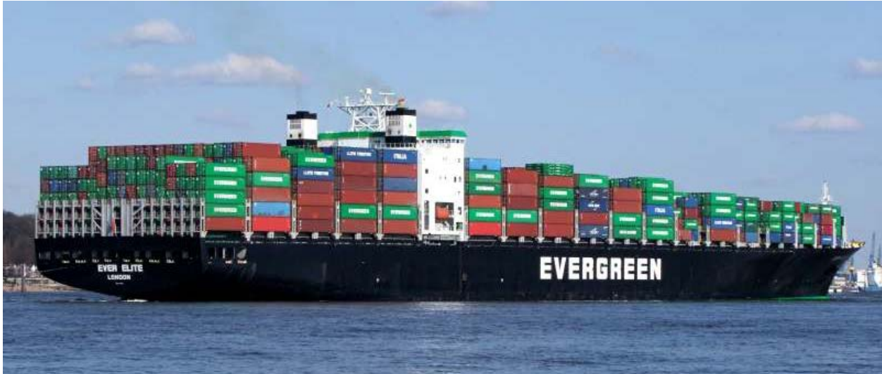
Figure 2-3: The container ship Ever Elite (IMO 9241281), 75,898 DWT, 981 ft. long, about 6,000 TEU [16].
