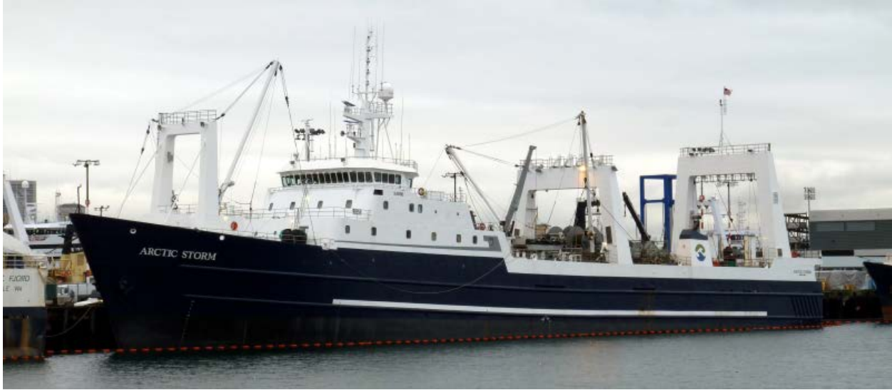
Figure 2-12: The commercial fishing trawler Arctic Storm (IMO 8720113), 2,638 DWT, 334 ft. long [16].
