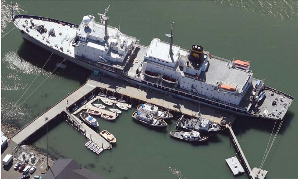
Figure 4-20: The Training Ship Golden Bear berthed at the California Maritime Academy in Vallejo, CA (image from Google). Ample spaces at the stern and just aft of the stack are on-board location options for a PEM fuel cell system.
