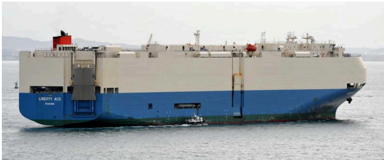
Figure 2-1: The auto carrier Liberty Ace (IMO 9293650), 19,106 DWT, 656 ft. long [16], with a capacity of approximately 6,400 average-sized cars. The asymmetric stern and ramp for loading/discharging vehicles is a typical feature of vehicle carriers.
