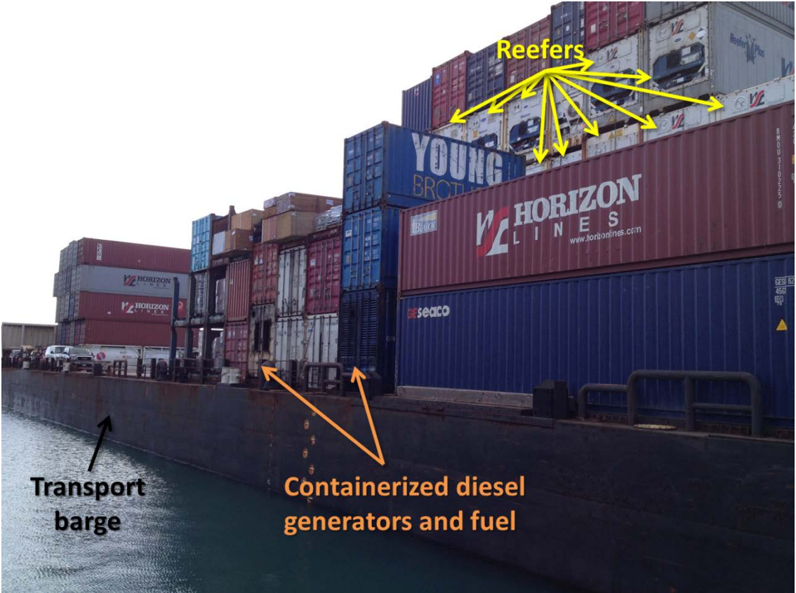
Figure 3-7: Transport barge loaded with containers. The refrigerated containers (“reefers”) are kept running with containerized diesel generators that are loaded and discharged with the reefers.
