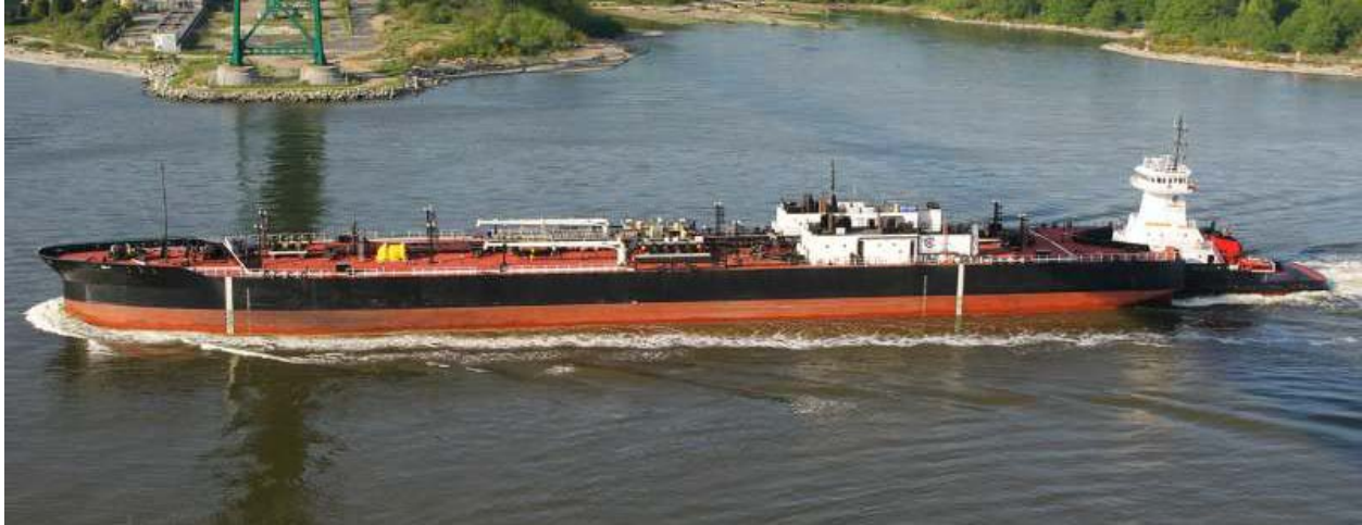
Figure 2-9: The articulated tug-barge Coastal Reliance (IMO 9271119) [16]. The V-shaped notch where the tug joins with the barge can be seen just in front of the white wheelhouse at the stern.
