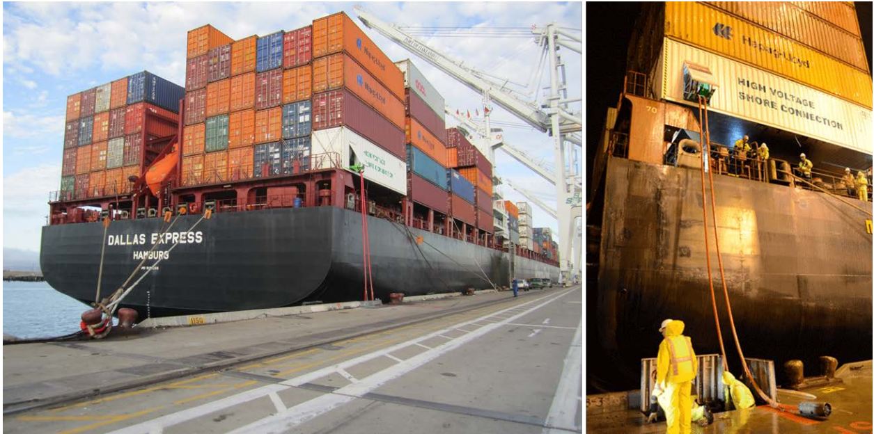
Figure 2-14: Hapag-Lloyd's Dallas Express using shore power at the Port of Oakland. The ship-side connectors and cables are housed in a special shipping container at the stern on the starboard side (white container at the bottom corner of the container stack). Left-side picture from [36], right side picture from [37].
