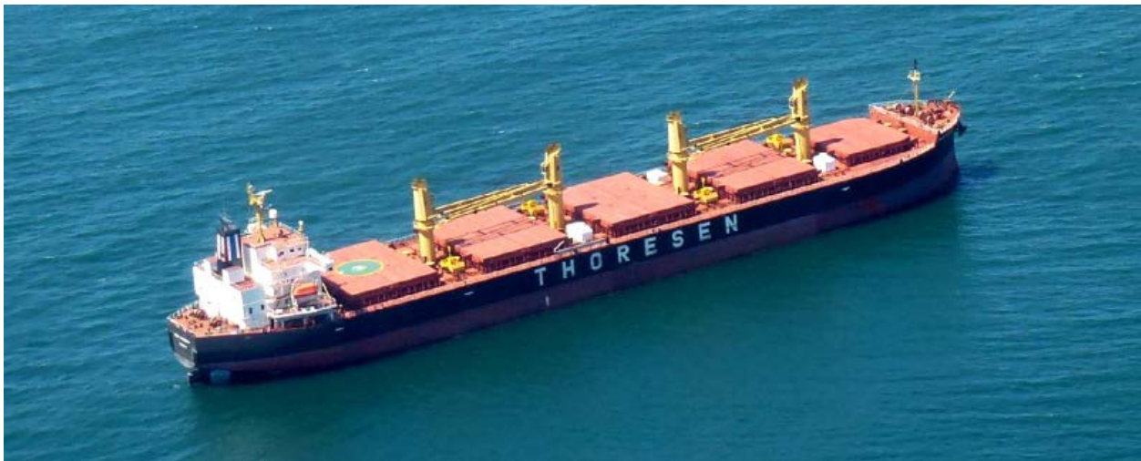
Figure 2-7: The break-bulk carrier Thor Friendship (IMO 9424601), 54,123 DWT, 623 ft. long [16].
