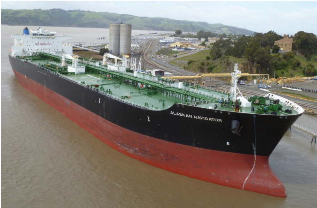
Figure 2-5: The crude oil tanker Alaskan Navigator (IMO 9244673), 193,048 DWT, 945 ft. long.
