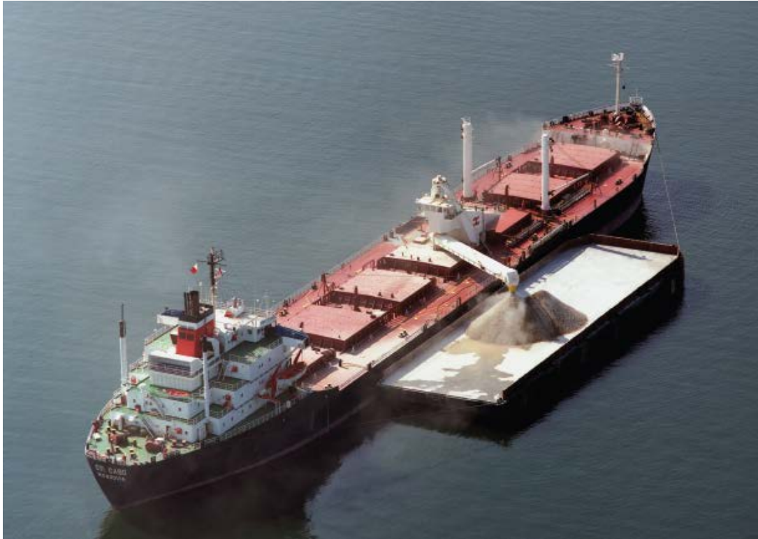
Figure 2-6: The self-discharging dry-bulk vessel CSL Cabo (IMO 7117278), 13,364 DWT, 594 ft. long, discharging gypsum onto a barge alongside [26].
