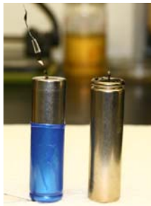
Before ARC After ARC Photo of the cell before & after Arc test
