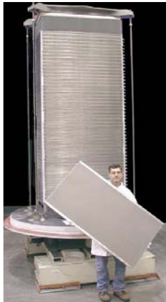
Cell Package and Stack
