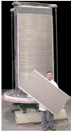
Cell Package and Stack
