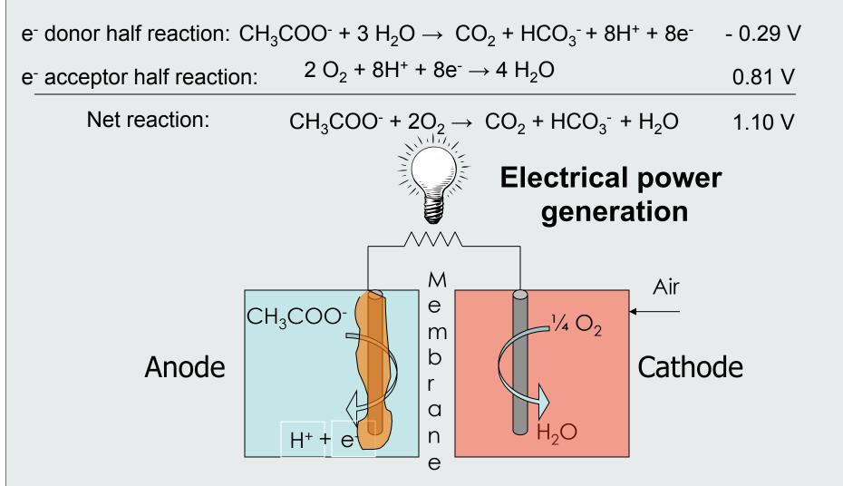
The reaction potential drives all biological, chemical, and electrochemical processes in MFC => typical recovered potentials are 0.3 - 0.6 V
