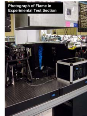
DLR-A Flame: Re_\delta = 15,200 Fuel: 22.1% CH 4 , 33.2% H 2 , 44.7% N 2 Coflow: 99.2% Air, 0.8% H 2 O Detailed Chemistry and Transport: 12-Step Mechanism (J.-Y. Chen, UC Berkeley)
