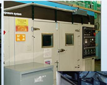
Environmental chamber for durability due to weather variations & freeze (at NREL's OTF)
