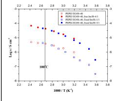
•Conductivity of fixed Imidazole polymer equal to the conductivity of the polymer doped with free imidazole solvent. •Relative concentration of Imidazole to acid group is critical. •Increase conductivity by optimization of tether length, acid/base concentration, nature of the acid group (Fluoroalkylsulfonylimides vs. Alkylsulfonate) and by control of the morphology to promote Grotthuss proton transfer.
