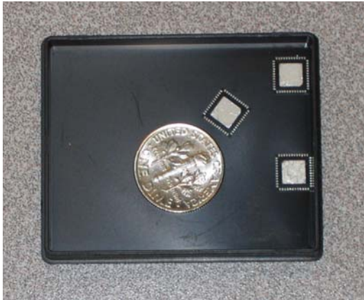
Three gate driver ICs in CDIL44 package in comparison with a dime
